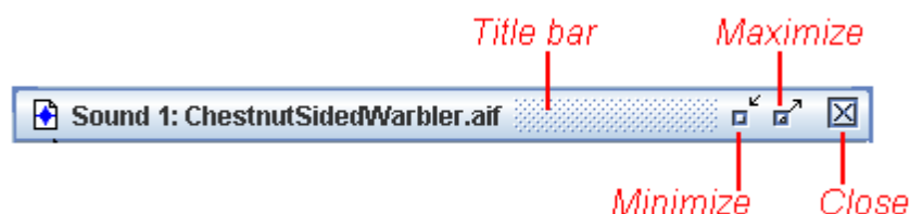
Figure 3.3. The title bar, with controls to resize and close a sound window. The title bar is also the anchor for moving the sound window.
