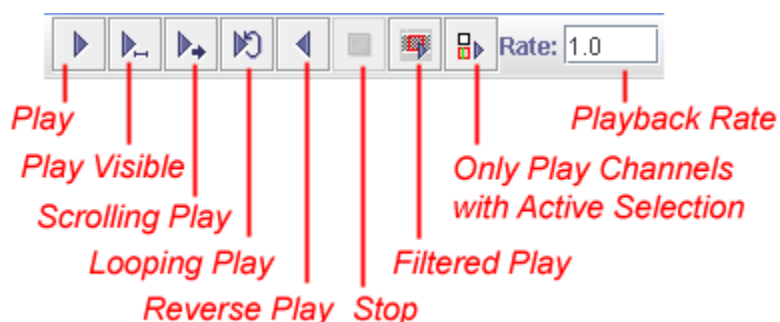
Figure 1.6. The playback controls in the play toolbar.
